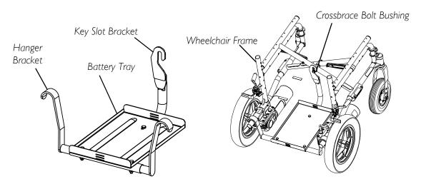
FIGURE 11.4 Installing/Removing Battery Tray
